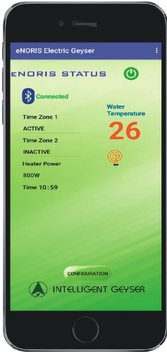
4. Electric heater is turned 'ON'
